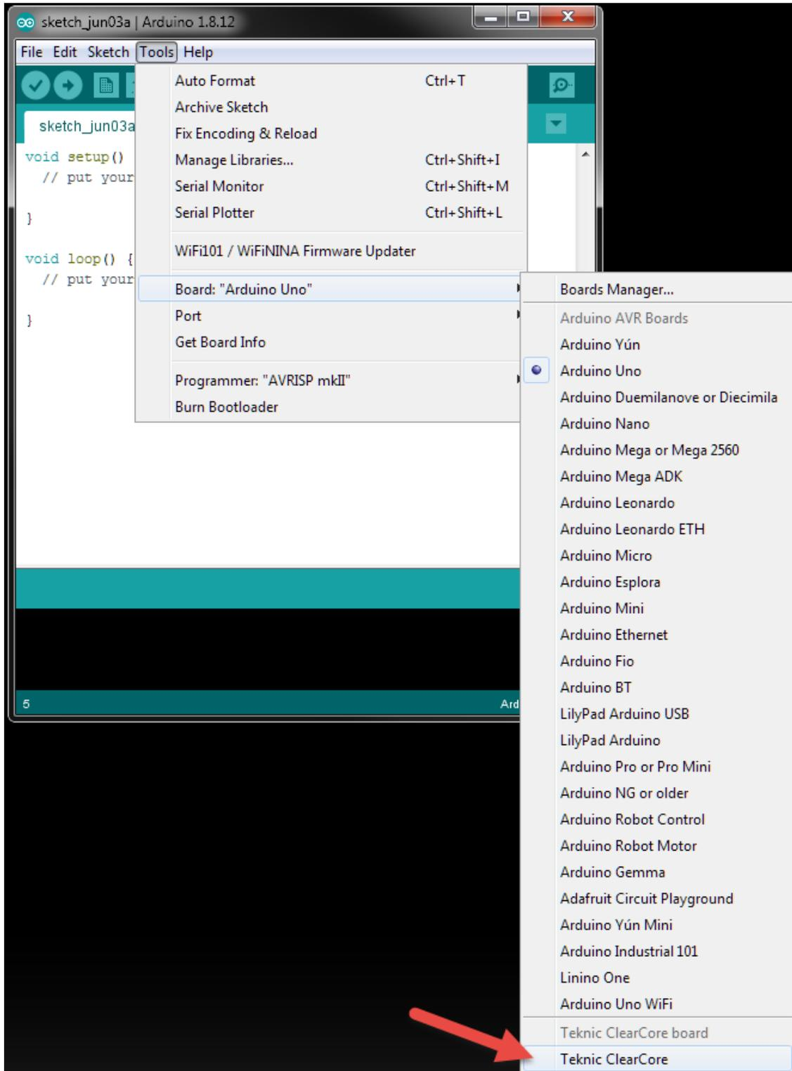
6) Supply power to your ClearCore (see [ClearCore User Manual](#) for detailed power information) and connect the ClearCore to your PC using a USB cable. Once connected, select Tools > Ports. Select the port named "Teknic ClearCore", e.g. "COM 11 (Teknic ClearCore)". Your COM port number may be different.
