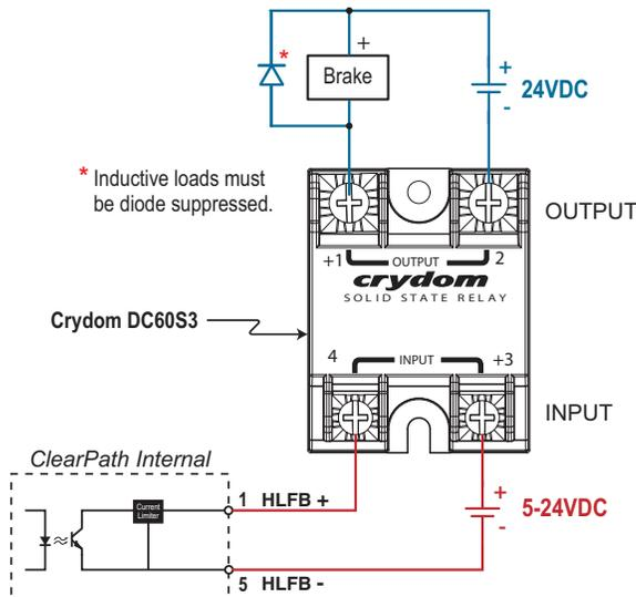
**HLFB circuit controlling an SSR / brake setup**
