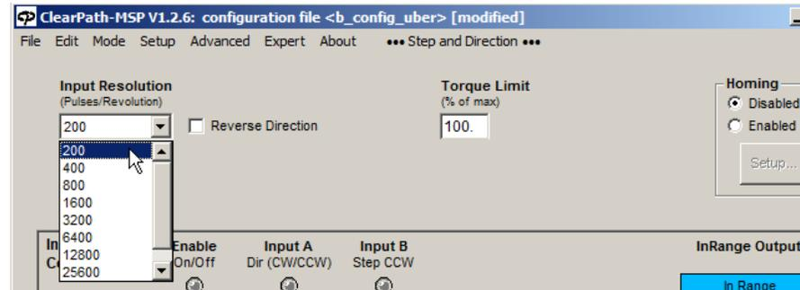
*With the above Input Resolution setting, it takes only 200 step pulses to make this [800 count] motor rotate one full revolution.*
