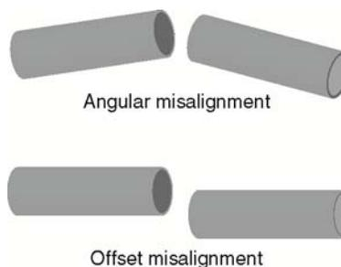
Some couplings are more forgiving of misalignment than others, but in general, misalignment will cause undesired vibration/noise, shortened bearing life, and even broken motor shafts.
