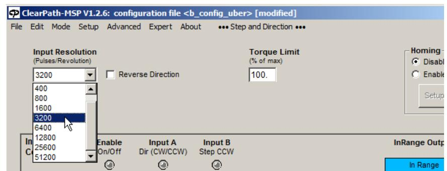
*With the above Input Resolution setting, it takes 3200 step pulses to make this [800 count per rev.] motor rotate one full revolution.*
