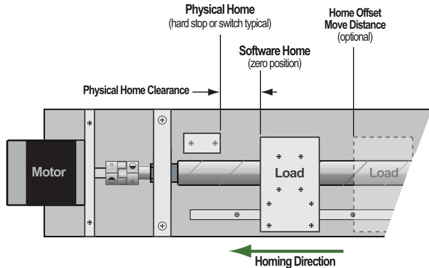
**Physical Home** - Physical Home is the position of a mechanical hardstop or home sensor. When the Physical Home is encountered, e.g. a homing switch is actuated, the position is recorded, and the ClearPath motor stops and moves away towards the final offset position.
