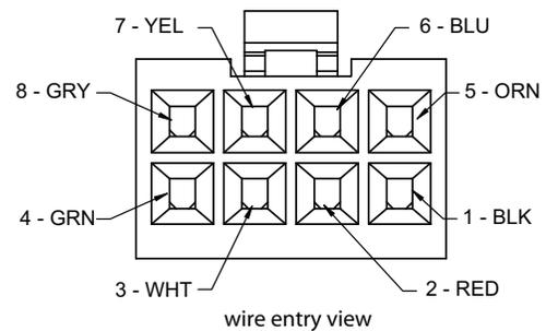
**POWER CABLE: CPM-CABLE-PWR-MM660**
