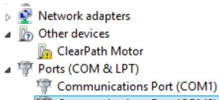
Right-click the "ClearPath Motor" device and select "Update Driver Software". If target PC has an internet connection, use the "Search Automatically...." option to update the driver. If *no internet connection* is available, use the "Browse my computer..." option and point to the following local folder:
